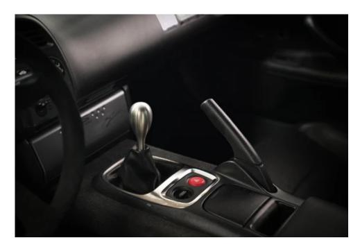
5. Align your Renegade Titanium E-brake button to the receiver rod and tighten by turning clockwise. The button needs to only be firmly tightened by hand, no pliers necessary. This completes your install.
