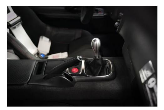
3. This is where you cover the button with the microfiber cloth if you are trying to preserve the OEM button. Get a firm grip on the OEM brake button with your pliers and turn counter clockwise. The button is seated deep, so keep loosening it all the way until you can remove with just your fingers.
